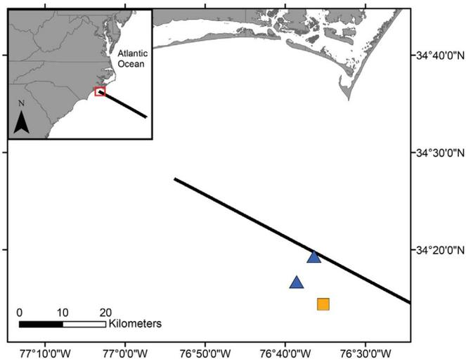
**Fig. 1.** Track of seismic survey vessel (black line) relative to three monitoring reefs on the inner continental shelf of NC: two outfitted with hydrophones (blue triangles) and one with video camera (orange square).
