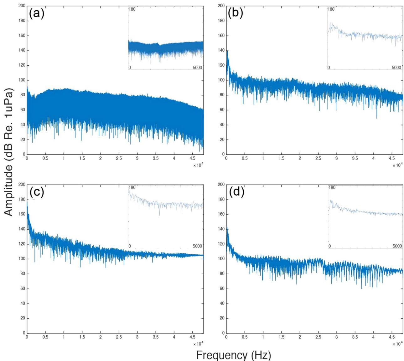
**Fig. 2.** Acoustic signatures of A) ambient noise and B-D) noise from seismic airgun shots on reef 0.7 km from closest approach of seismic surveying vessel: B) 22.2 km from reef before closest approach; C) 0.7 km from reef showing the seismic shots just prior to shots that overloaded our instruments; D) 19.6 km from reef following closest approach. Insets depict 10 Hz – 5 kHz range of low frequency.
